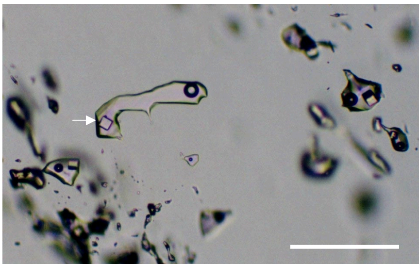
Fig. 1 Photomicrograph of fluid inclusions in quartz crystal from Kawahage. The inclusions contained saline water, vapor bubbles, and cubic NaCl crystal (white arrow). Scale bar is 200 \mu\text{m} .
