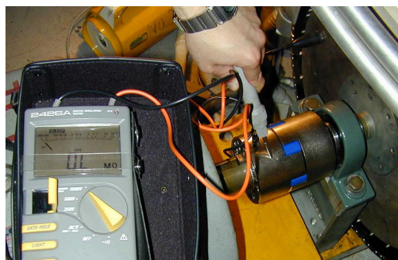
Fig.7 A photograph of the chain-motor coupling. It is made of Hytrel developed by DU PONT-TORAY Co., Ltd. We selected it in order to insulate between the motor and the sheave.
