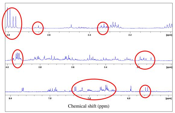
Figure 4-7  $^1\mathrm{H}$  NMR spectrum of SE in  $\delta\mathrm{H}$  2.00-2.80, 3.00-4.00 and 6.00-8.00 ppm
