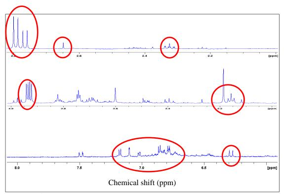
Figure 4-8 <sup>1</sup>H NMR spectrum of SCE in δH 2.00-2.80, 3.00-4.00 and 6.00-8.00 ppm
