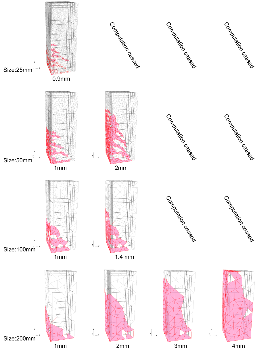
Fig. 6. Distribution of cracked solid elements for indicated step of posing displacement boundary condition.
