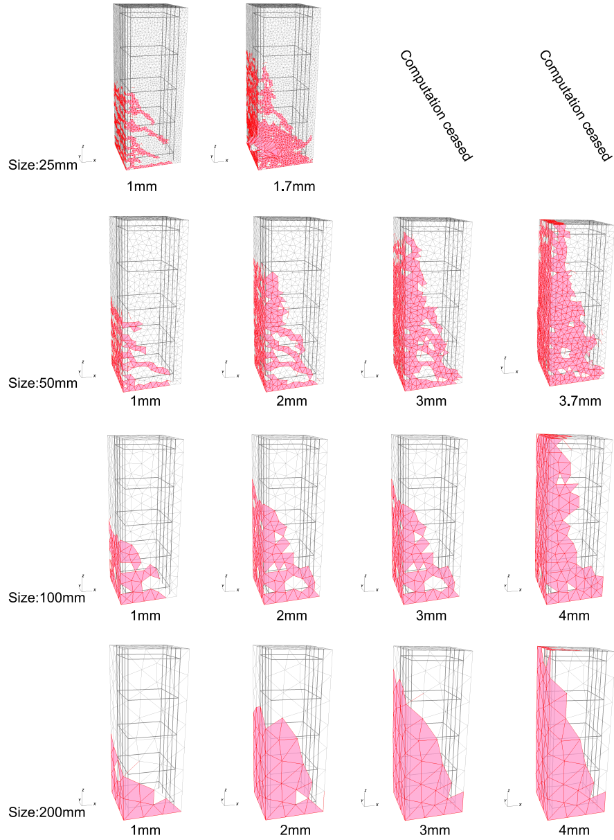
Fig. 9. Distribution of cracked solid elements w/o re-contacting for indicated step of posing displacement boundary condition.
