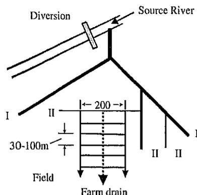
Fig. 4 Standard Layout of Irrigation and Drainage System in Japan.
