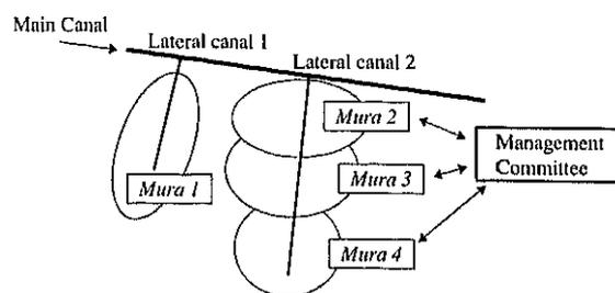
Fig. 5 Establishment of Management Committee for Common Lateral Canal: *Mura* is a basic unit for irrigation management in Japan.
