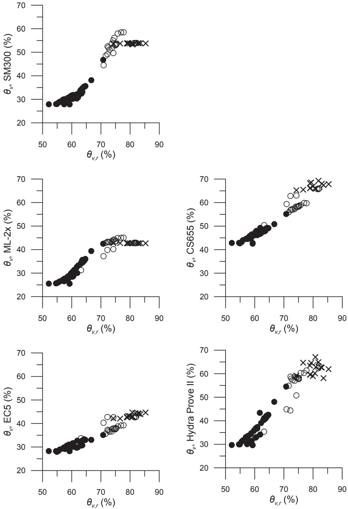
Fig. 2 Relation between the  $\theta_v$  values measured by the five sensors and the reference  $\theta_{v,r}$  values from the weight measurement. Closed circles indicate those for bulk EC  $\leq 1.5$  dS/m, open circles for  $1.5 < \text{bulk EC} \leq 2.5$  dS/m, and crosses for  $2.5 \text{ dS/m} < \text{bulk EC}$ .
