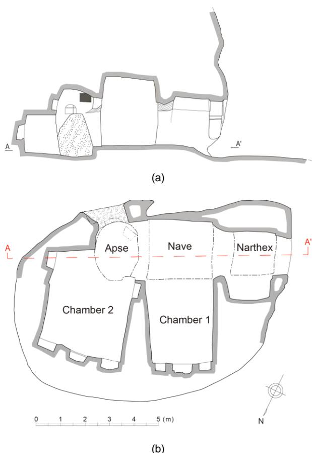
**Figure 3:** The drawings of the Üzümlü Church: a) East-west (AA') section; b) Ground floor plan.
