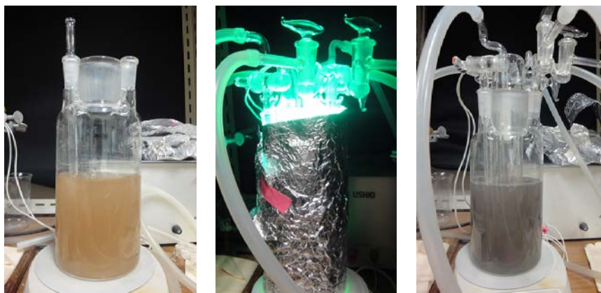
(a) Before irradiation, (b) under UV irradiation and (c) immediately after the 3 h irradiation.
