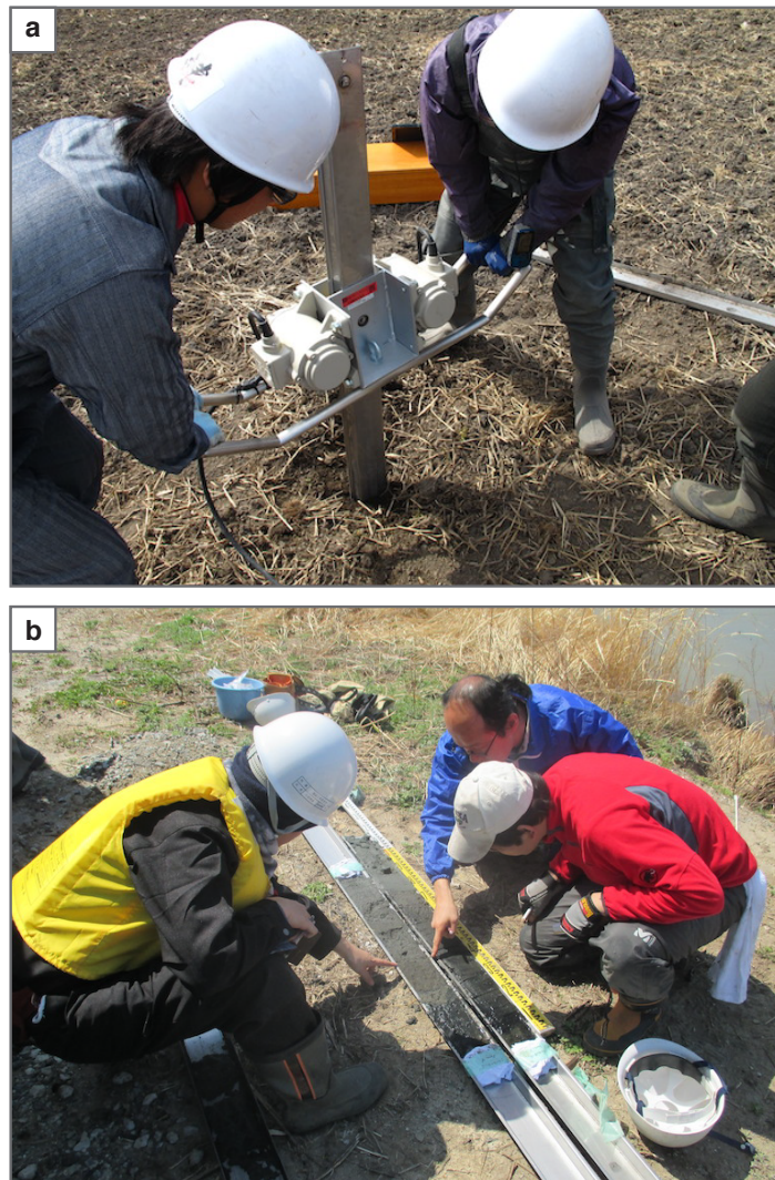
Fig. 3-1. Sample collection. (a) Collection of sediment sample using handy geoslicer. (b) Observation of sediment sample collected by handy geoslicer.
