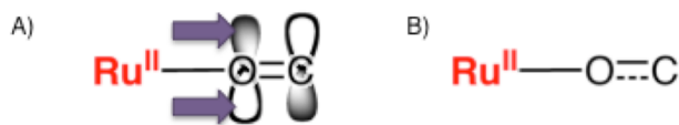
Figure 2-24. (A) \pi -back donation from ruthenium(II) center to \pi^* orbital on the carbonyl bond of PQQTME ligand and (B) weakened double bond character of the carbonyl bond by the \pi -back donation from ruthenium(II) center.
