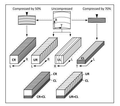
**Figure 1** Structure and fiber alignment of uncompressed beam (UR and UL), compressed beam (CR), reinforcement plate (CL) and composite beams (UR+CL and CR+CL).
