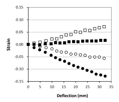
**Figure 8** Surface strains of compressed wood as a function of deflection under four-point bending.
