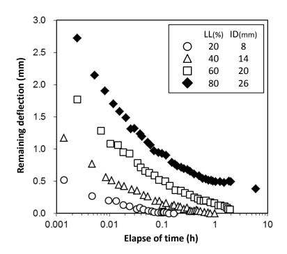
**Figure 11** Changes in remaining deflection of composite beam ( $CR+CL_{0.1}$ ) with elapsed time after the removal of load.
