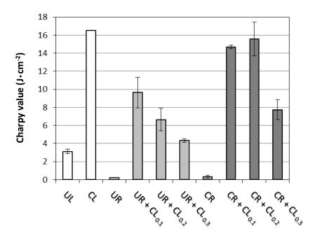
Figure 7 Average Charpy values of tested beams.
