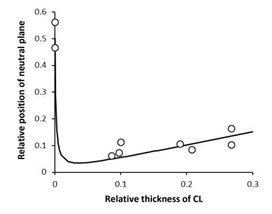
**Figure 9** Relative position of neutral plane of composite beams (CR+CL) under four-point bending plotted against the relative thickness of CL. Solid curve indicates the results of calculation based on the average Young's moduli of CR and CL.
