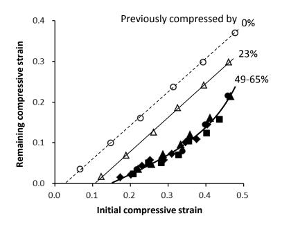
**Figure 3** Effects of initial compressive strain on the remaining compressive strain of cedar wood.
