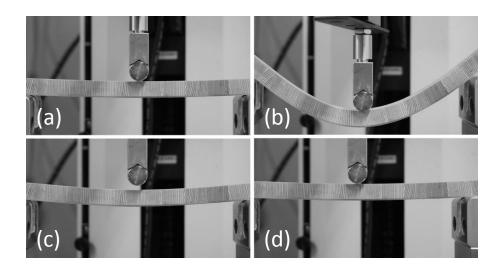
**Figure 10** Viscoelastic shape recovery of composite beam (CR+CL<sub>0.1</sub>) after the removal of load.
