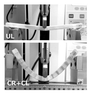
**Figure 4** Failure of uncompressed beam (UL) at small deflection and ductile bending of composite beam (CR+CL<sub>0.1</sub>) under three-point bending test.
