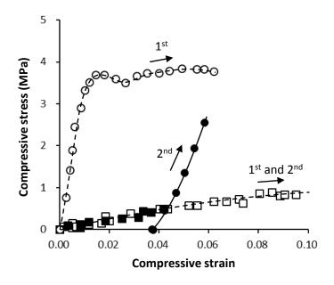
**Figure 2** Compressive stress-strain diagrams of cedar wood. Circles, uncompressed wood; squares, previously compressed by 50%; open plots, first compression; filled plots, second compression.
