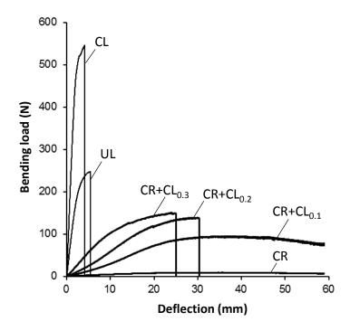
Figure 5 Load-deflection curves of tested beams.
