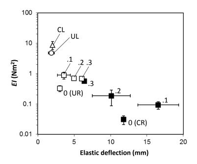
**Figure 6** Flexural rigidity (EI) of tested beams plotted against elastic deflection. Open circle, uncompressed wood in L direction (straight grain); open triangles, compressed wood in L direction (flat grain); open squares, composite beam (UR+CL); filled squares, composite beam (CR+CL).
