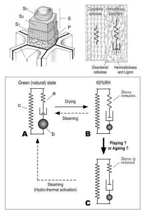
**Fig.1.** A viscoelastic model to explain the drying stress and its relaxation.
