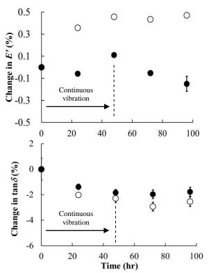
**Fig.2.** Change in E' and  $\tan \delta$  plotted against the elapse of time.  $\bigcirc$ , Dry specimen tested at 60%RH;  $\bullet$ , steamed specimen tested at 100%RH.
