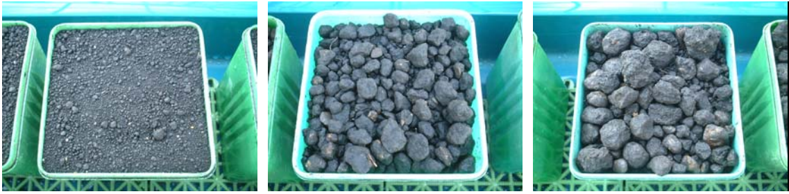
Fig. 20 Soil surface with sieved soil in plastic container. A container was filled with clay to 3 cm from the top, and initial watering was conducted. Sieved soils of three particle sizes were mixed with SETVI seeds, and placed into the pre-prepared containers up to their maximum capacity. (Left < 5 mm, Center 5 mm to 15 mm, Right > 15 mm)
