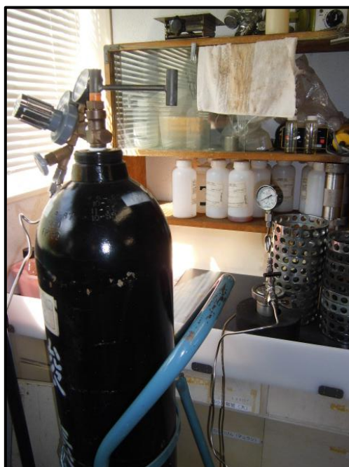
Figure A1.3 Charge oxygen gas under 0.35-0.50 MPa at room temperature
