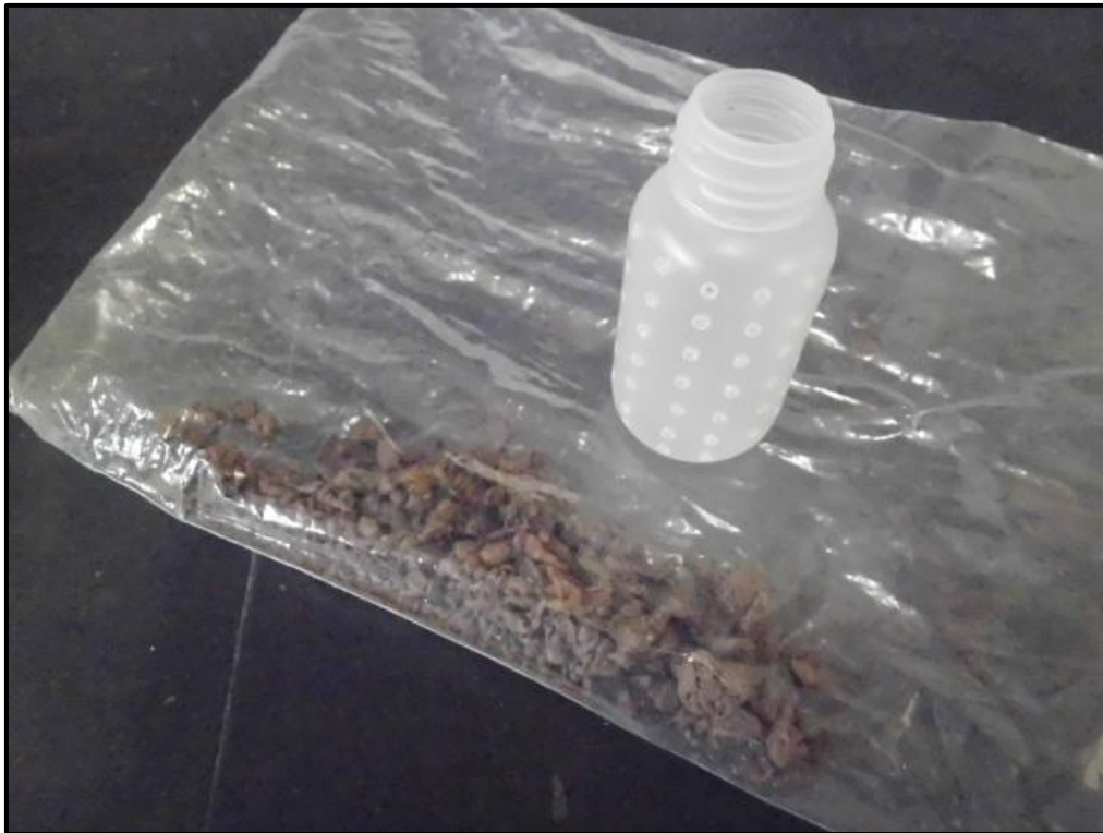
Figure A1.1 Put pulp in polyethylene plastic bag and make pulp into small particles (diameter 5-10 mm)
