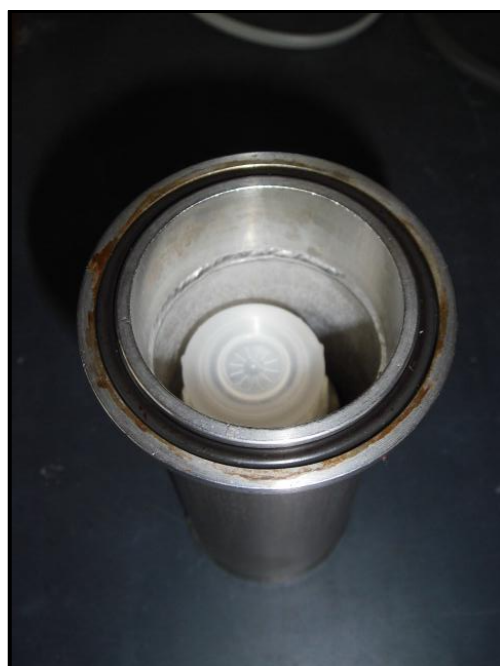
Figure A1.2 Put pulp in a polypropylene plastic bottle, and then put the plastic bottle into the reactor
