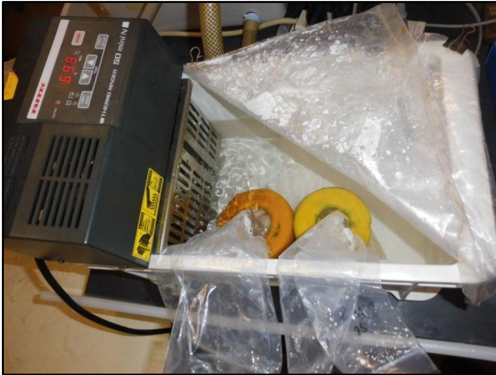
Figure A4.2 Put the sample inside the water-bath, and make sure that the position of the sample is submerged under the water
