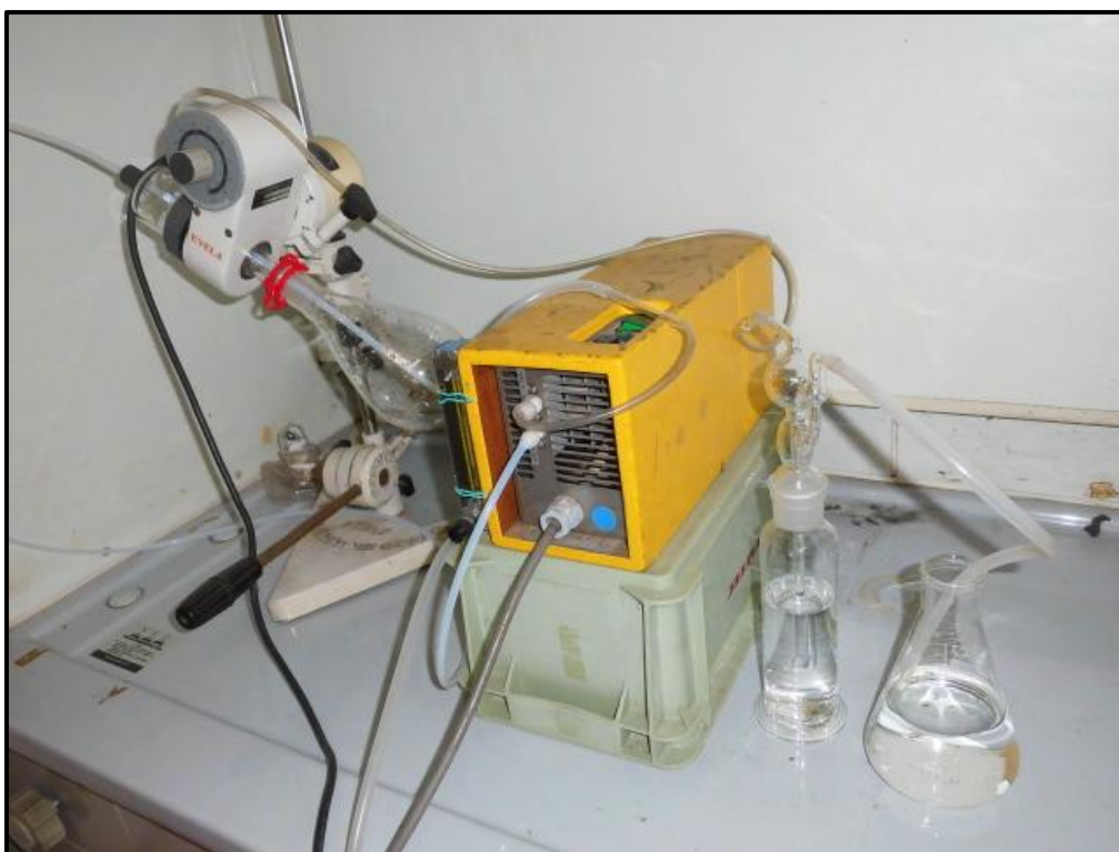
Figure A3.4 Set of ozone bleaching equipment excluding O 2 gas tube
