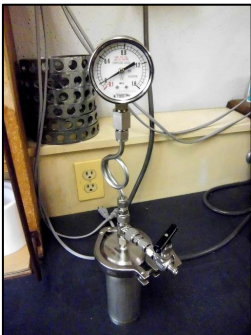
Figure A1.3 Charge oxygen gas under 0.35-0.50 MPa at room temperature
