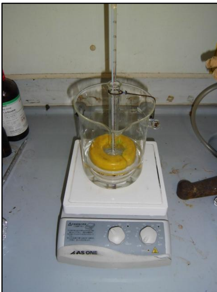
Figure A2.2 The position of the 100 mL flask inside the beaker
