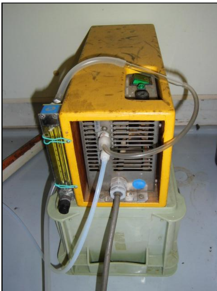
Figure A3.1 Ozone generator set with O 2 gas flow at 0.4 L/min
