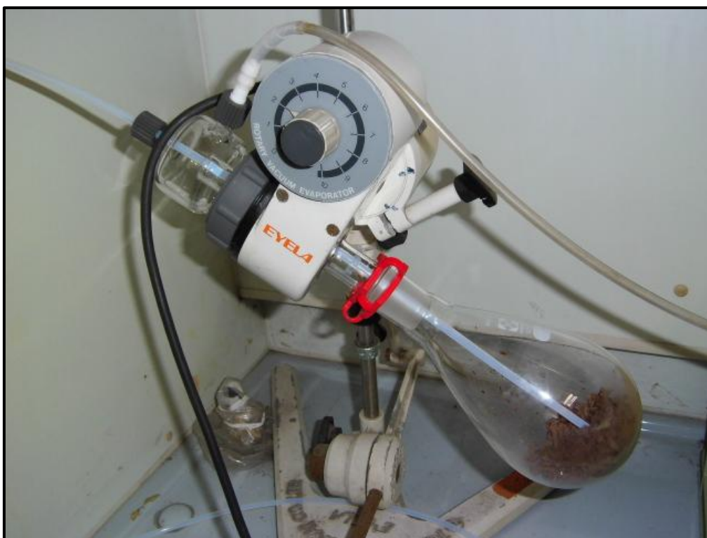
Figure A3.2 Pulp sample put in the eggplant flask and set in the rotating reactor
