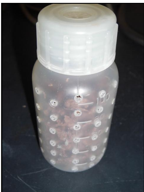
Figure A1.2 Put pulp in a polypropylene plastic bottle, and then put the plastic bottle into the reactor
