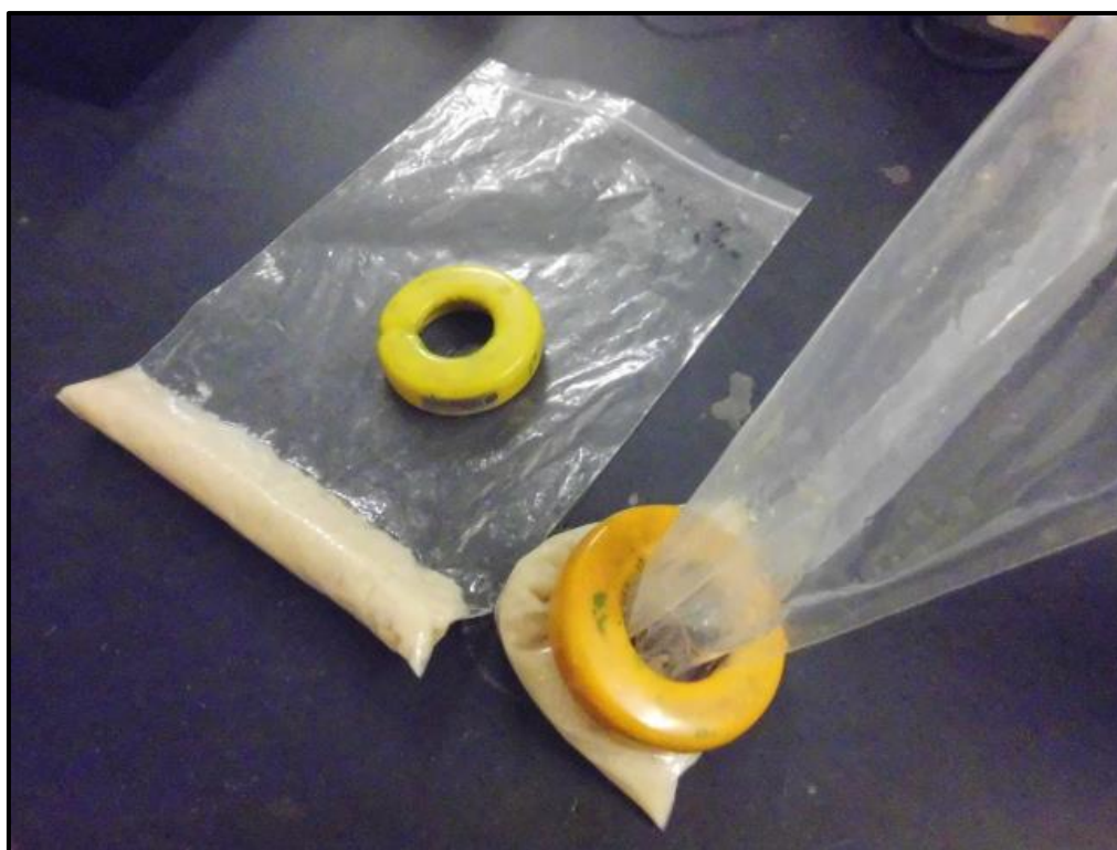
Figure A4.1 Put a mixture of sample and chemicals in a polyethylene bag, and remove the air in the bag, and then put a weight
