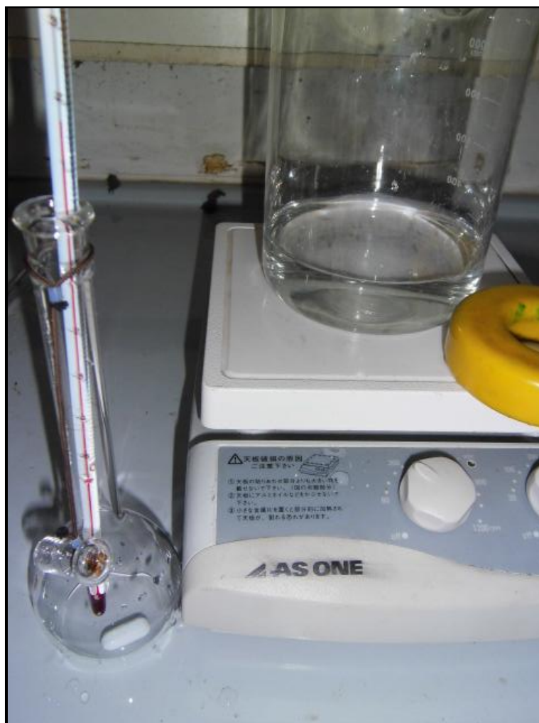
Figure A2.1 The position of the thermometer and the small stirrer bar inside the 100 mL volumetric flask
