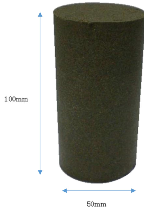
Fig. 2.5 Finished specimen for conventional triaxial tests
