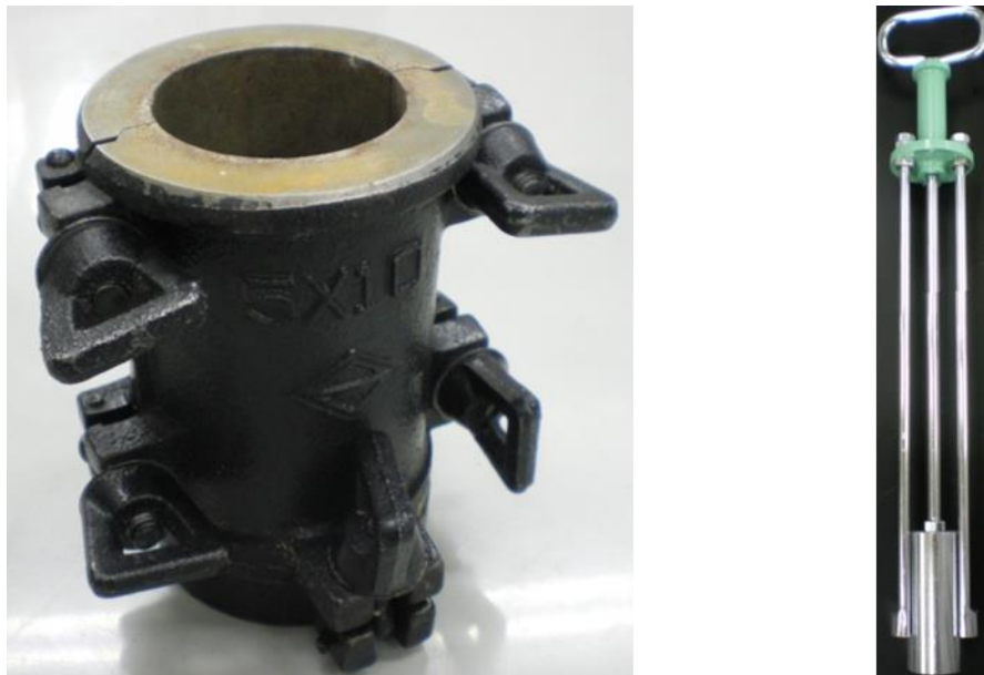
Fig. 2.4 Mold (left) and rammer (right) for compaction
