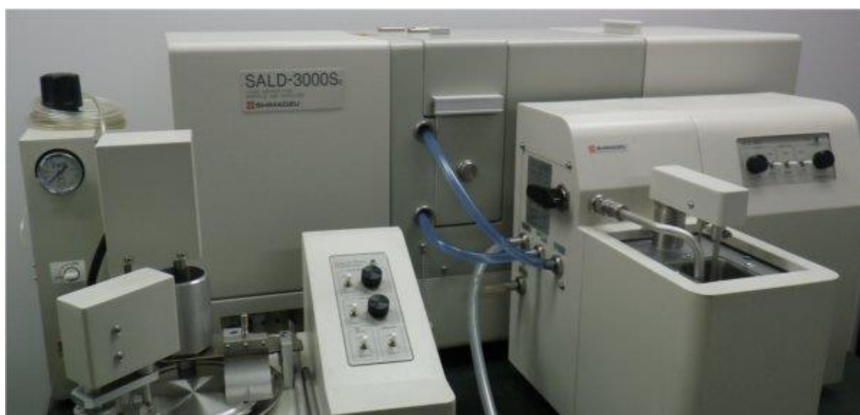
Fig. 2.2 Laser diffraction particle size analyzer (SALD-3000S; Shimadzu Co., Ltd.)
