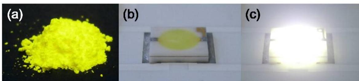
Figure 7-17 (a) new yellow phosphor; (b) as-prepared LED; (c) LED in operation.
