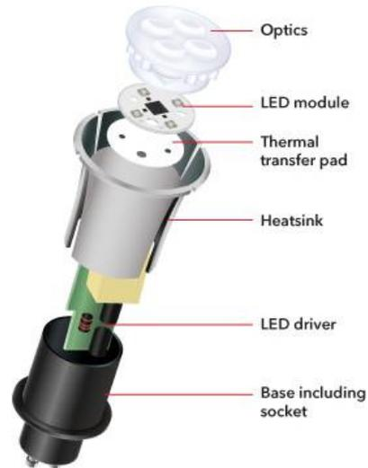
Figure 2-19 Schematic illustration of LED light bulb.<sup>43</sup>
