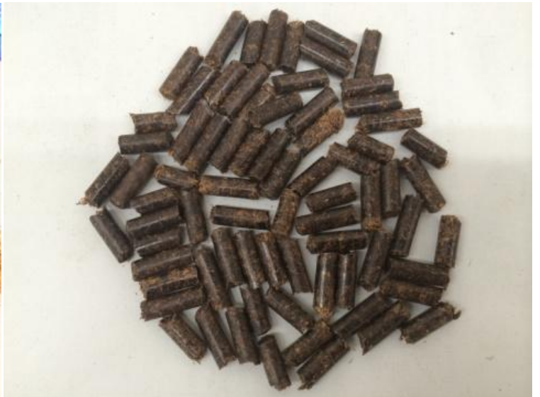
EFB Pellet (0.5 cm diameter and 1.5 cm length)
