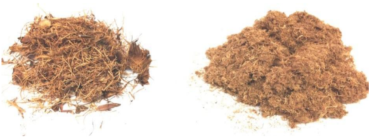
Photo 3-2 Unrefined EFB fiber (left) and TMP-refined and hot air-dried pulp (right)
