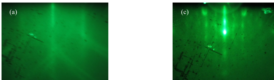
Fig. 51(a) 1 \times 1 RHEED pattern after thermal cleaning of Si on SOI at 590 °C, observed along \langle 11-2 \rangle azimuth and (b) RHEED pattern after RDE growth along Si[11-2] azimuth.
