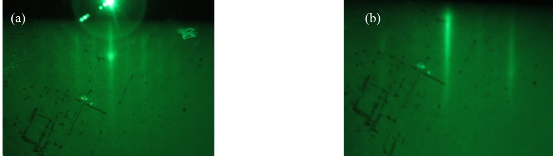
Fig. 52(a) RHEED patterns after MBE growth along Si[11-2] and (b) along Si[1-10] azimuth.
