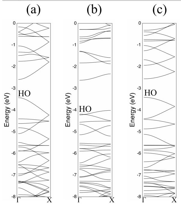
**Fig. 5.** Electronic energy bands of coronene polymers with (a) six-membered, (b) five-membered, and (c) four-membered rings. HO denotes the highest branch of the valence band. Energies are measured from that of the vacuum level.
