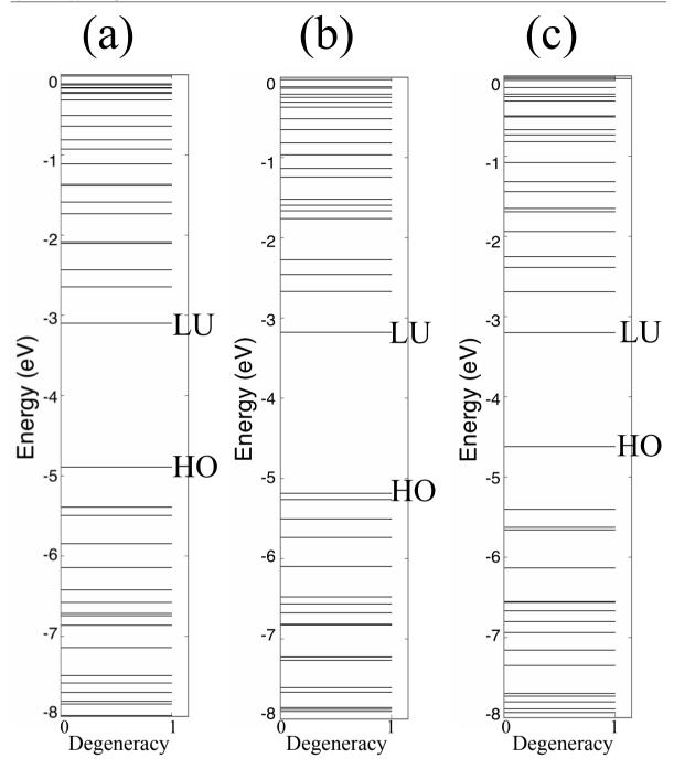
**Fig. 2.** Electronic structure of dicoronylenes molecules for isomers with (a) six-membered, (b) five-membered, and (c) four-membered rings. Energies are measured from that of the vacuum level.
