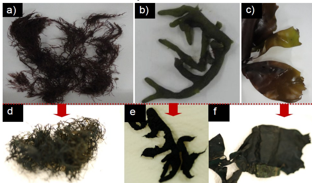
Figure 1. (a): Gelidium , (b): Codium fragile , (c): Grateloupia elliptica Holmes. (d): Bio-composite of PANI/ Gelidium (PANI- Gelidium ), (e): PANI/ Codium fragile (PANI- Codium ), (f): PANI/ Grateloupia elliptica Holmes (PANI- Grateloupia ).
