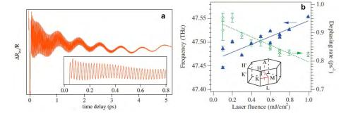
Figure 17. (a) Transient EO reflectivity change at pump power of 50 mW. The inset shows an enlargement of the trace to show the high-frequency modulation. (b) Laser fluence dependence of the dephasing rate and the frequency of the coherent  $E_{2g2}$  phonon obtained from a fit to an exponentially damped oscillator function. The lines are to guide the eyes. Inset shows the Brillouin zone of graphite.
