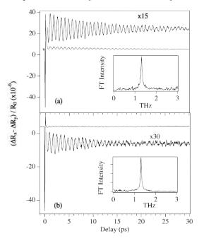
**Figure 10.** Time-resolved EO reflectivity change obtained for graphite before (a) and after irradiation with  $8 \times 10^{13} \text{He}^+/\text{cm}^2$  (b). The insets show the Fourier transforms of the time-domain signals (after ref. [39])
