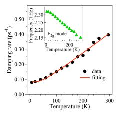
Figure 21. Decay rate of the  $E_{2g}$  mode together with the frequency (inset) as a function of the lattice temperature. The solid line represents the fit to the data using equation (13) with  $\Gamma_0 = 0.06 \text{ ps}^{-1}$ .
