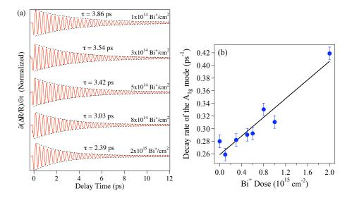
Figure 7. (a) The time derivatives of the TR signal.  $\tau$  is the decay time of the coherent  $A_{1g}$  mode deduced by curve fitting with a damped harmonic oscillator. The dashed curve corresponds to the guide for a single exponential decay. (b) The decay rate of the coherent  $A_{1g}$  mode obtained by inverting the decay time  $\tau$  as a function of Bi<sup>+</sup> dose. The solid line corresponds to the fit of the data with equation (1) using  $\tau_{anharmonic} = 3.86$  ps.
