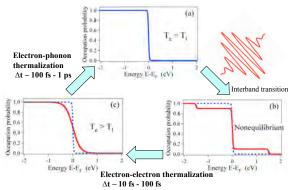
Figure 13. Dynamics of photo-generated electrons in metals. (a) Occupation probability of electrons in thermal equilibrium, where the electron temperature  $T_e$  equals to the lattice temperature  $T_l$ . (b) Occupation probability of electrons in nonequilibrium just after the irradiation of femtosecond laser pulses. (c) Occupation probability of electrons after electron-electron thermalization, where  $T_e > T_l$ .
