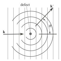
Figure 1. Schematic of phonon-defect scattering; scattering of an incident phonon of wavevector  $\mathbf{k}$  by a defect. The scattered wave is spherical and the wavevector  $\mathbf{k}'$  represents a set of transitions from  $\mathbf{k}$  to  $\mathbf{k}'$ .  $\theta$  is the angle between  $\mathbf{k}$  and  $\mathbf{k}'$ .
