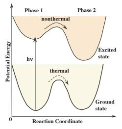
**Figure 24.** An illustration of the mechanism for the laser induced nonthermal phase transition. The dashed arrow indicates phase change (from phase 1 to 2) occurring for thermodynamical equilibrium, while the solid arrow indicates phase change (from phase 1 to 2) occurring for nonthermal process.
