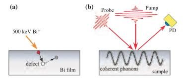
**Figure 4.** Experimental techniques. (a) Bi<sup>+</sup> ion irradiation into Bi thin films to introduce lattice defects. (b) Schematic of the pump-probe reflectivity measurement. The stronger pump pulse generates coherent phonons in solids, while the weaker probe pulse detects the change in the reflectivity through the photodiode (PD).
