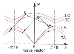
**Figure 3.** Anharmonic phonon decay processes. The TO phonon (a) decays into LA and TA phonons, while the LO phonon (b) decays into LA and TA phonons at slightly different wave vectors. The horizontal broken line represents the Umklapp process, where the wavevector of the TA phonon is created outside the first Brillouin zone.
