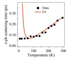
Figure 15. The temperature dependence of the electron-phonon thermalization time  $(\tau_q)$ . The closed squares are experimental data while the solid curve is a fit to the data with the TTM model, described by equation (10).
