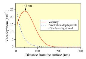
**Figure 6.** The damage profile of the Bi film with Bi<sup>+</sup> ion irradiation, compared with the penetration depth profile of the femtosecond laser used in the experiment.
