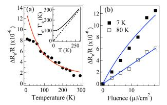
Figure 16. (a) The amplitude of the fast electronic transient as a function of temperature. Inset shows the corresponding initial  $(T_e$  - dashed) and final  $(T'_e$  - solid) electronic temperatures as a function of temperature. (b) The amplitude of the fast electronic transient versus the pump fluences at the two typical temperatures. The solid curves are the fit to the data using equation (12).
