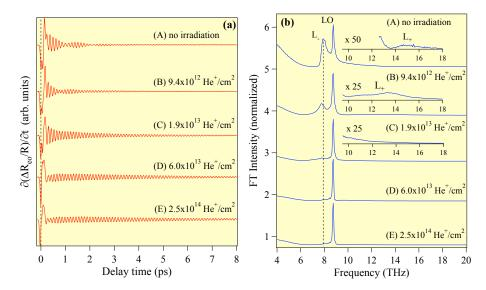
**Figure 9.** (a) The time derivatives of the EO signal for n-GaAs obtained at 300 K for various He<sup>+</sup> doses. (b) FT spectra obtained from time domain data in (a). The dotted line shows the peak frequency of the TO mode for the unirradiated sample, indicating that the  $L_{-}$  mode locates at almost the TO frequency because the  $L_{-}$  mode is phonon-like at  $(n_{dop} + n_{exc}) \sim 2 \times 10^{18}$  cm<sup>-3</sup>.
