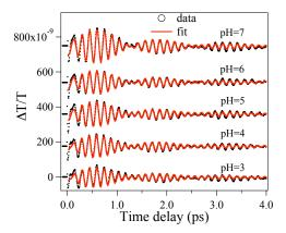
Figure 27. Time domain signal from the coherent RBM in SWCNT obtained by subtracting carrier responses from the transient transmission  $\Delta T/T$  at various pH values. The solid lines represent the fit to the time-domain data with a linear combination of the damped harmonic oscillators.
