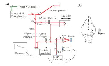
Figure 5. Experimental techniques used for the case of GaAs. (a) Pump-probe optical set-up based on Electro-optic (EO) sampling mode. (b) EO reflectivity change induced by the light field (E) on the (001) surface, which is detected by the difference in the reflectivity between  $R_{\perp}$  and  $R_{\parallel}$ .
