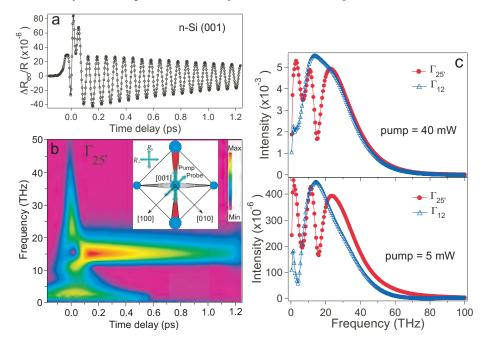
Figure 11. (a) Transient EO reflectivity change for Si(001) in  $\Gamma_{25'}$  geometry. (b) Continuous wavelet transform (CWT) of (a). Insets define the polarization of the pump and probe light relative to the crystalline axes. (c) Slices of CWT spectra in (a) at zero delay for two different geometries,  $\Gamma_{25'}$  and  $\Gamma_{12}$  (after ref. [34]).
