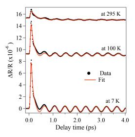
**Figure 14.** TR signal observed for Zn at 7 K, 100 K, and 295 K. The closed circles are experimental data, the solid curve is the fitting with equation (6).
