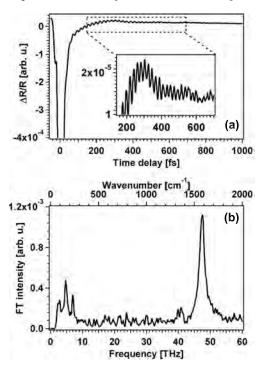
**Figure 18.** (a) Time-resolved transient reflectivity of SWCNTs. The inset represents the enlargement panel to show the coherent phonon oscillation. (b) FT spectrum of the time-domain datum in (a).
