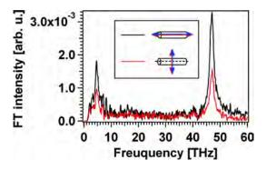
**Figure 19.** FT spectrum of the time-resolved reflectivity of SWCNTs with different polarization set-ups, as shown in the inset.
