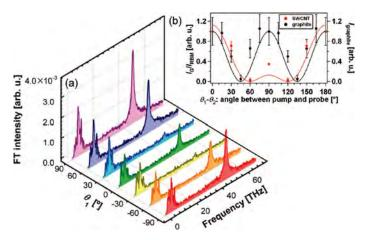
Figure 22. (a) FT spectra obtained from time-domain  $\Delta R/R$  signal as the functions of the frequency and the polarization angle  $\theta_1$ . (b) The ratio of the intensity of the coherent phonon spectra of the G-mode to the RBM as the function of the angle between the pump and probe beams.
