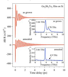
**Figure 26.** The TR signal observed in amorphous and crystalline  $Ge_2Sb_2Te_5$  films at 295 K. The insets represent FT spectra obtained from the time-domain data.
