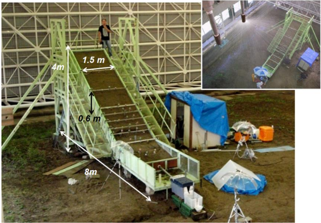
Fig. 4.2 A large flume experiment and artificial rainfall in NIED.
