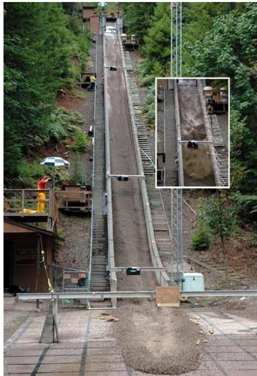
Fig.1.3 Experimental debris flow descending U.S. Geological Survey debris-flow flume
