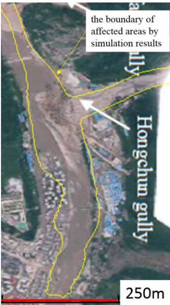
Fig.5.43 The comparison simulation results with actual damage in term of affected areas
