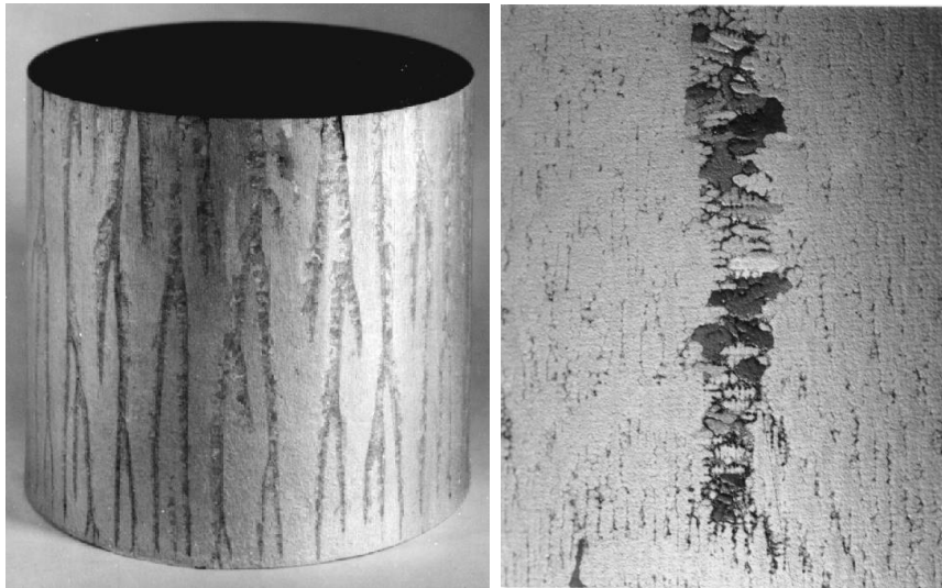
Figure 1.2 The freckle defects in single-crystal Ni-based superalloy.
