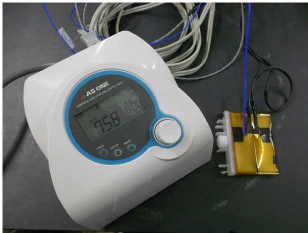
Fig. 2.4 Ink cartridge wrapped with film-type heater.
