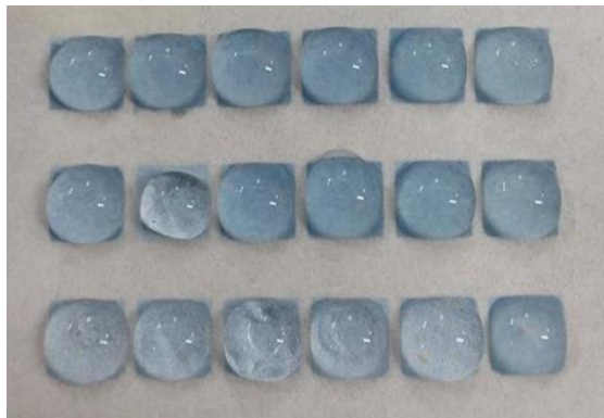
Fig. 4.6. CA hydrogel on hydrophilic areas on hydrophilic/hydrophobic patterned paper.
