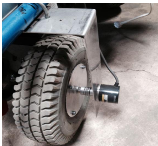
Fig. 6.6 Incremental rotary encoder in velocity control system
