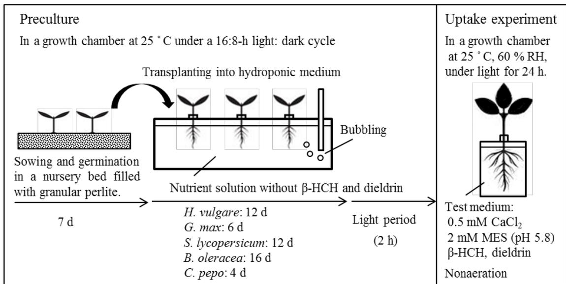
**Figure 1 A schema of time-course of uptake experiment by several plants in hydroponic medium.**
