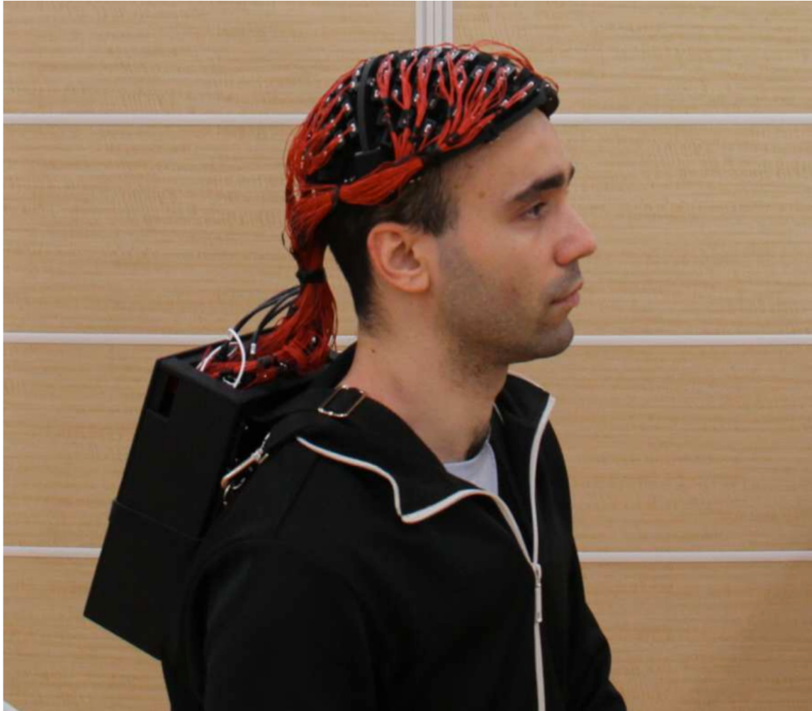
FIGURE 40 - COMPLETE WEARABLE ELECTRODE GRID WITH USER
