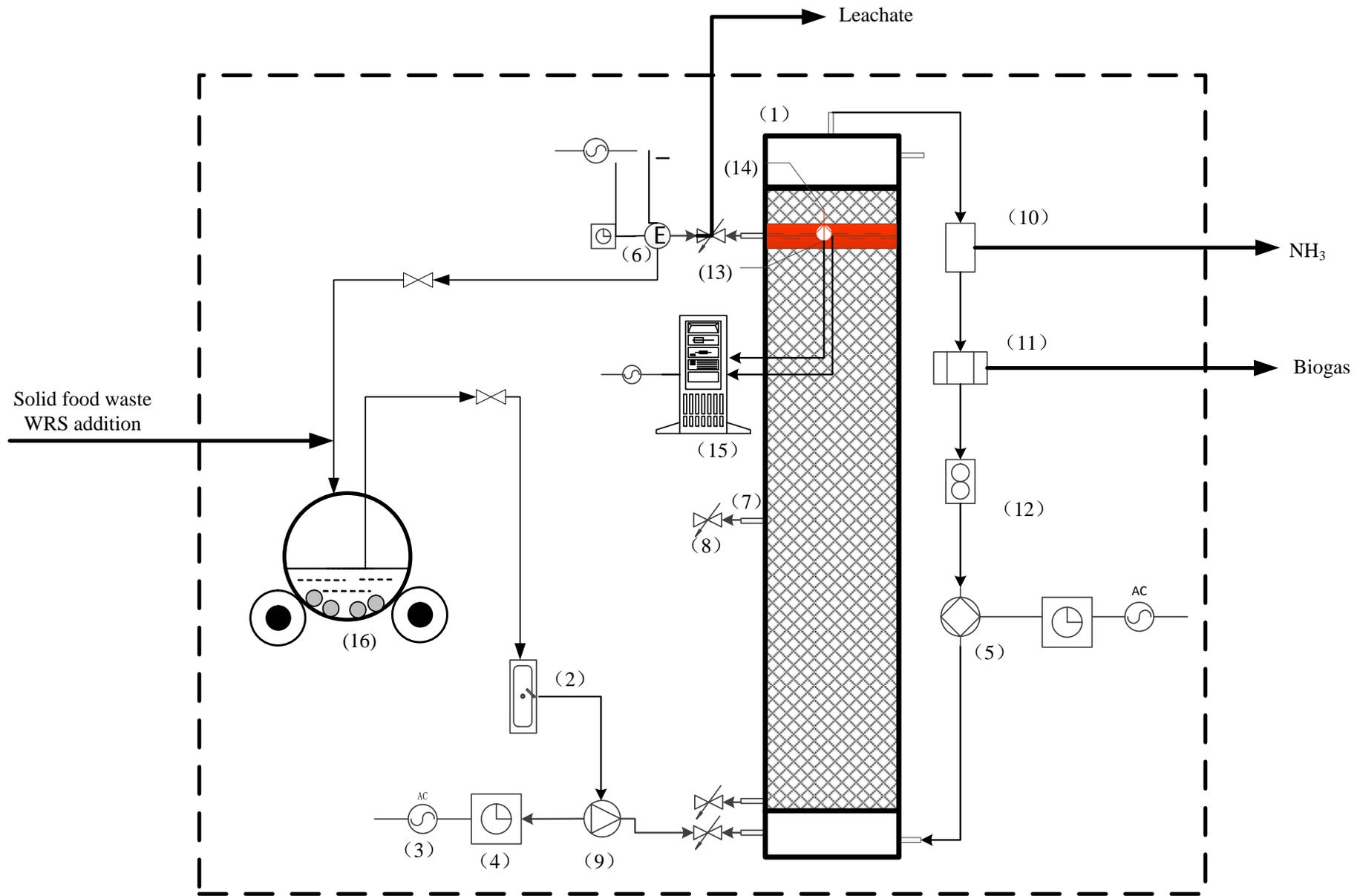
Fig. 5-1 The conceive for the combination system for the anaerobic fermentation of the solid and liquid food processing waste
