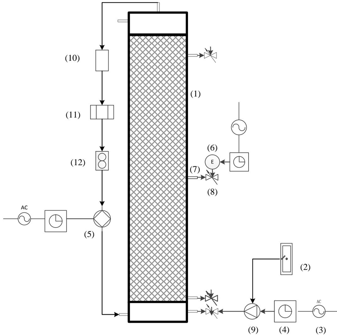
Figure 3-1 Scheme of the fixed bed reactor for ammonia production
