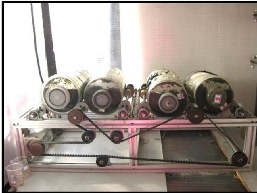
Figure 2-1 Apparatus for the simultaneous pretreatment and acidogenesis system for the solid food waste
