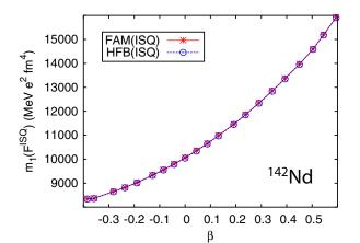
FIG. 2. (Color online) Energy-weighted sum rule of the isoscalar quadrupole operator in <sup>142</sup>Nd obtained in the HFB (solid line with asterisks) and FAM (dashed line with open circles) frameworks as a function of quadrupole deformation  $\beta$  for the constrained HFB solutions.
