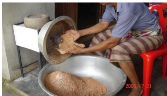
Figure 1.9 Milling a piece of sago trunk , Nayong , Trang Province.
