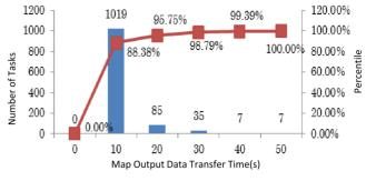
Fig. 7 Cumulative Distribution of map output data transfer time
