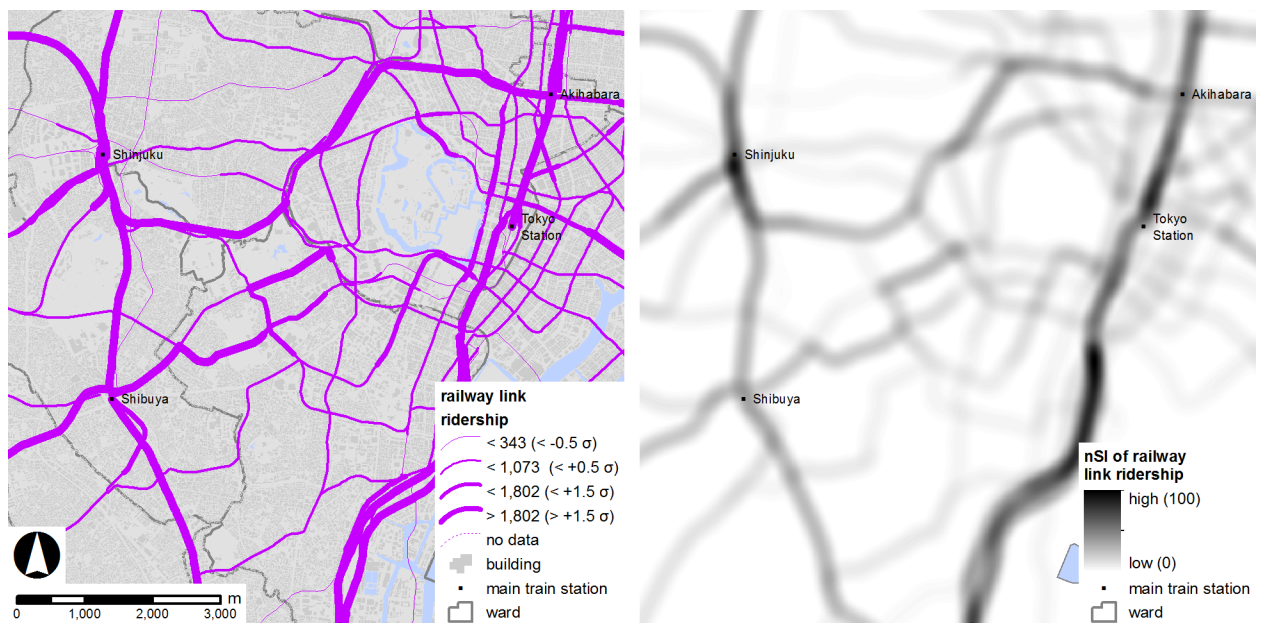
Figure 35: Comparison of the estimated railway link ridership (left) and the resulting raster surface representing the normalized spatial influence (nSI) (right) for a detail of the study area at 8am.
