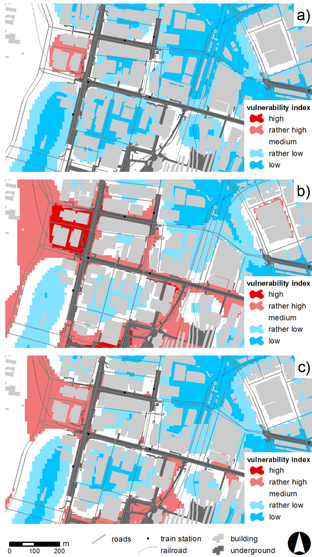
Figure 44: Raise of the vulnerability index as a result of single crowded buildings and building clusters in Marunouchi and Otemachi at a) 3am, b) 9am, and c) 7pm.
