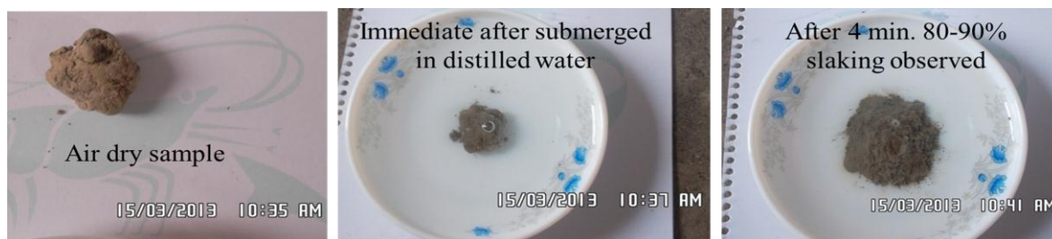
Figure 4.18 Slaking test for soil sample 3
