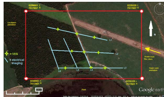
Figure 2 - Location geophysical survey.
