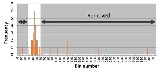
Fig. 7 Removing false matches using histogram of brightness gradient differences.
