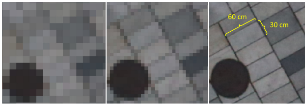
Fig. 21 Differences in appearance caused by spatial resolution: 12 cm/pixel (left), 6 cm/pixel (center), 1 cm/pixel (right).
