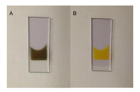
Fig. S7. Images of P-DFF films in oxidized state (A) and neutral state (B).
