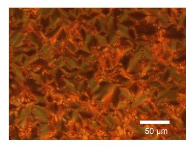
Fig. 4. POM image of fingerprint texture of blend cholesteric LC.
