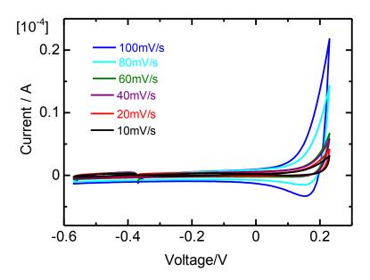
Fig. 12. CV curves of P-DFF film.
