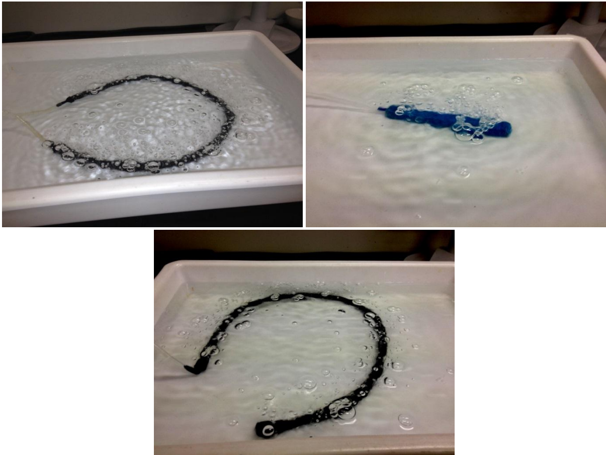
Picture 2-10 Test of diffusers operated at 1.0 \text{ L}\cdot\text{min}^{-1} air flow rate
