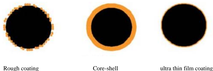
Fig. 1.6. Schematic of three types of surface coating with different techniques.
