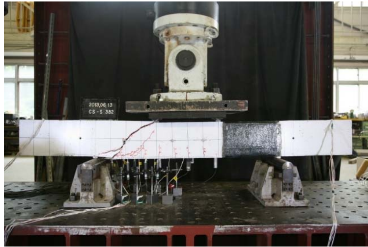
Fig. 2.9 (a) Failure mode of specimen CS-S
