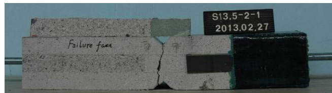
Fig. 4.4 (a) Typical failure faces of the specimens with small initial angles
