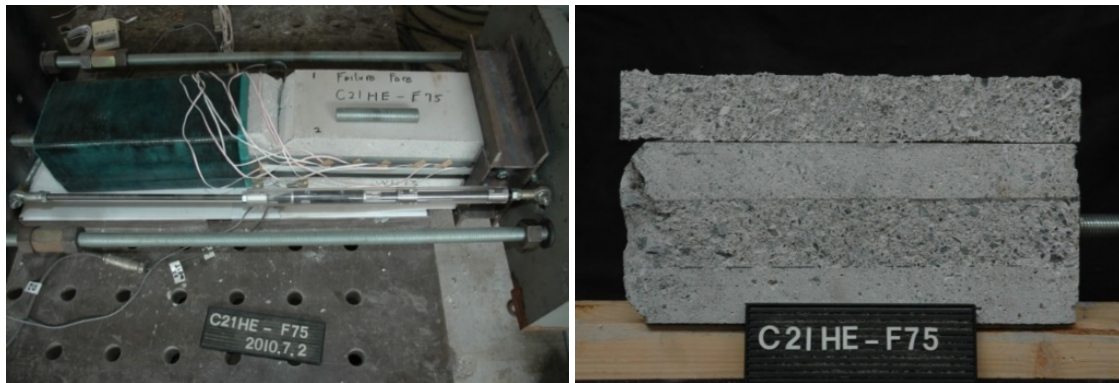
Fig. 3.12 Specimen C21HE-F75-C with a confinement jig and the failure surface
