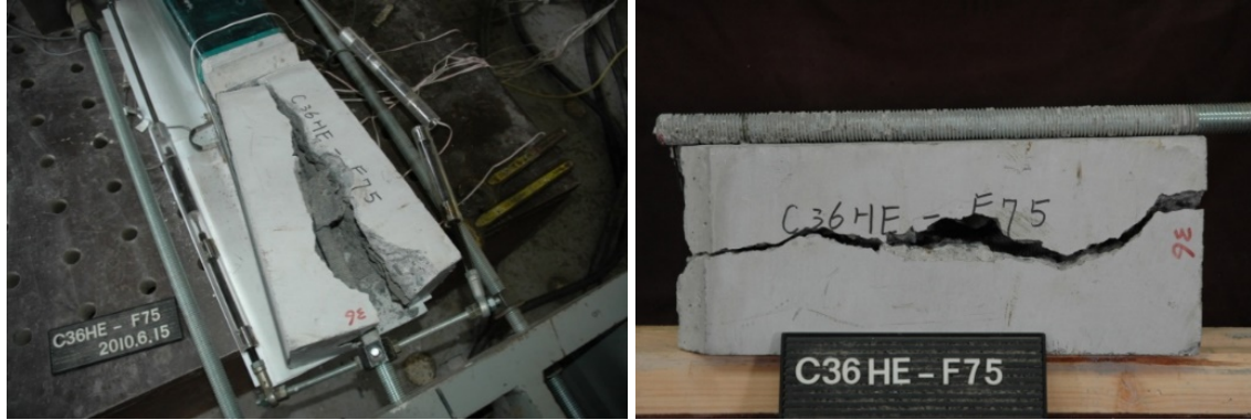
Fig. 3.11 Splitting failure of specimen C36HE-F75
