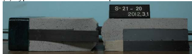
Fig. 4.4 (b) Typical failure faces of the specimens with large initial angles
