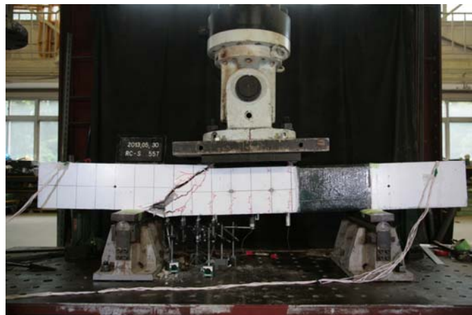
Fig. 2.6 Failure mode of specimen RC-S
