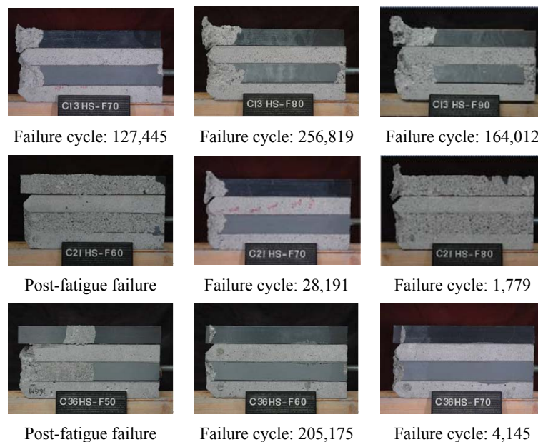
Fig. 3.13 Typical failure surfaces after fatigue loading
