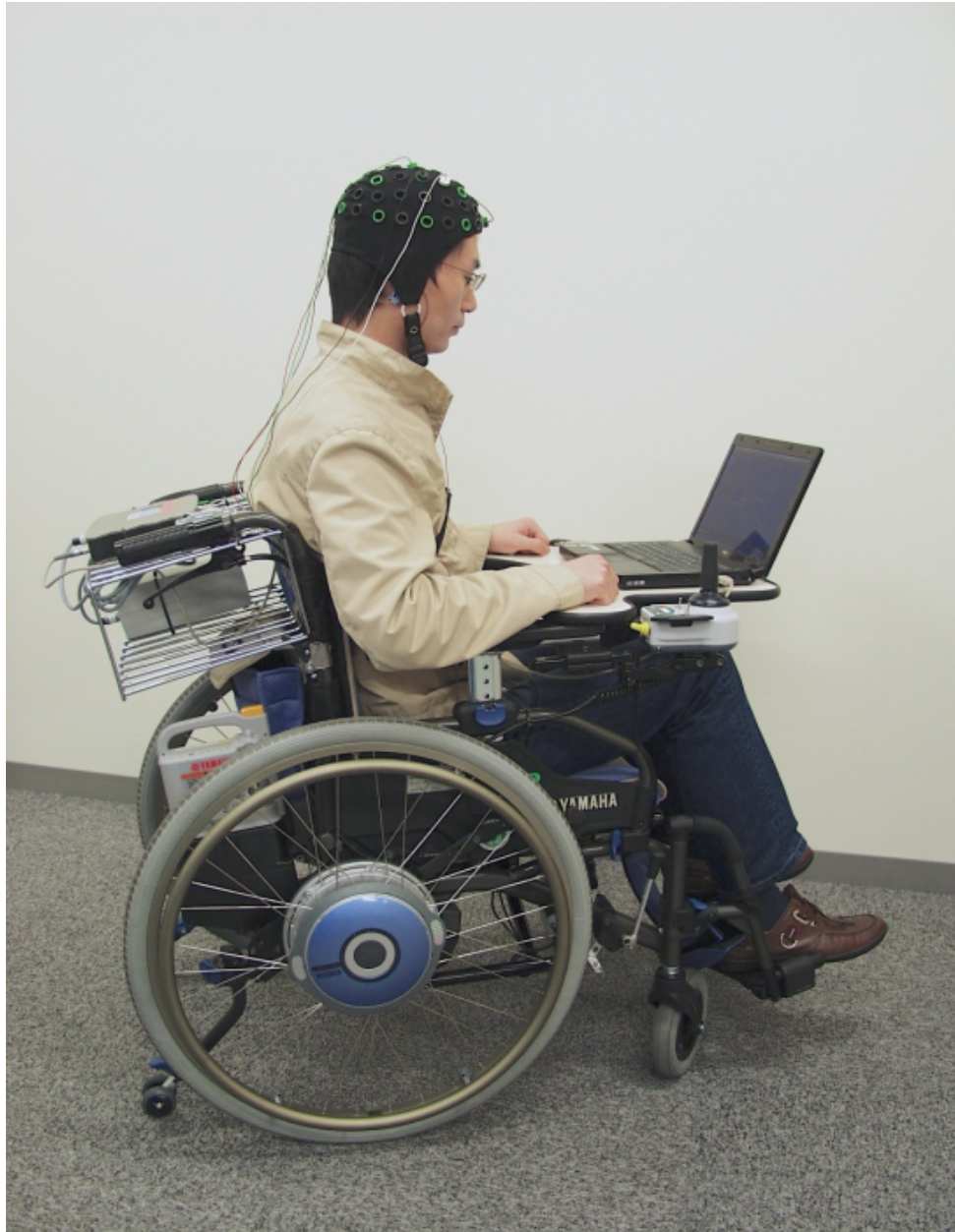
FIGURE 2.5: With the RIKEN's brain controlled wheelchair, the user continuously controls the velocity of the wheelchair by imagining left hand, right hand or both feet movements (Figure obtained permission)
