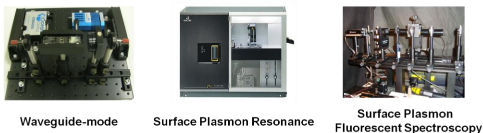
Figure 1.12. Sensing systems preferred to demonstrate the applications of PEG- b -polymers. All these sensors are operates based on the principle of Kretschmann configuration.
