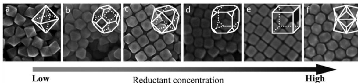
**Figure 2.** SEM images of well-faceted polyhedral Au nanocrystals. The shape and the concentration of ascorbic acid for each nanocrystal type were (a) octahedron, 0.6 mM; (b) truncated octahedron, 1.2 mM; (c) cuboctahedron, 1.4 mM; (d) truncated cube, 1.8 mM; (e) cube, 2.0 mM; and (f) trisoctahedron, 10 mM.
