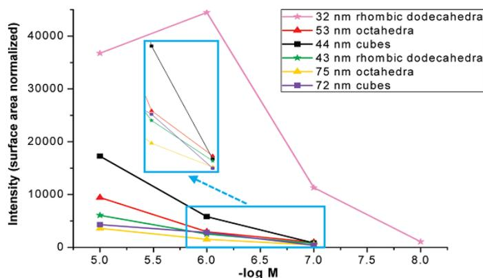
**Figure 4.** A plot of the total particle surface-area-normalized SERS intensities of the band at  $998\text{ cm}^{-1}$  versus thiophenol concentrations in the Au nanocrystal solutions. Data points at a  $1.0 \times 10^{-6}\text{ M}$  thiophenol concentration have been expanded to make their relative intensities visible.
