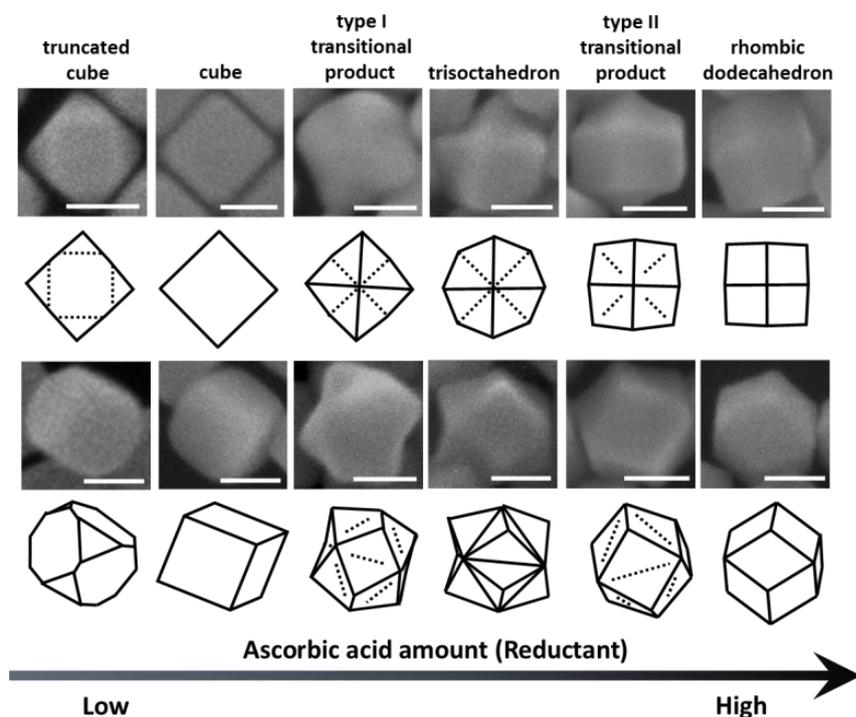
**Figure 1.** SEM images and the corresponding drawings showing the morphological evolution of the gold nanocrystals synthesized by varying the amount of ascorbic acid added to the reaction solution. Two different particle orientations are shown for each sample. All scale bars represent 50 nm.
