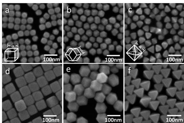
**Figure 3.** SEM images of (a, d) cubic, (b, e) rhombic dodecahedral, and (c, f) octahedral gold nanocrystals with edge lengths of (a) 44, (b) 32, (c) 53, (d) 72, (e) 43, and (f) 75 nm. Geometric models and edge lengths of these nanocrystals are also provided.
