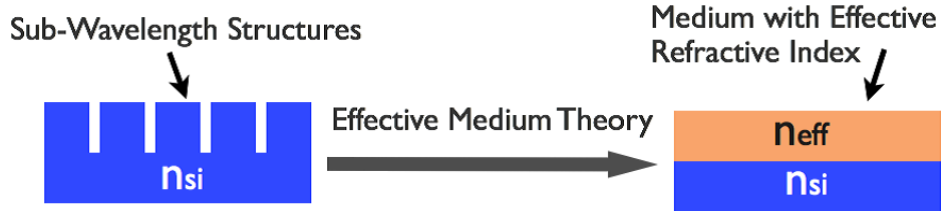
Figure 6.10: Cross-sectional view of the effective medium theory. A sub-wavelength structure can be regarded as a homogenous dielectric layer with an effective refractive index.
