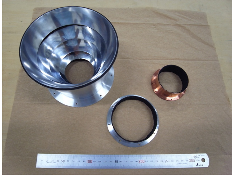
Figure 7.20: Photograph of the cold baffles. Left, center and right baffles correspond to the large 4 K nested baffle with reflective plates, small 4 K baffle and 1 K baffle, respectively. The 4 K baffles are made of aluminum. The 1 K baffle is made of oxygen free copper. The black parts of the inside of the baffles showed the absorber with a carbon black.
