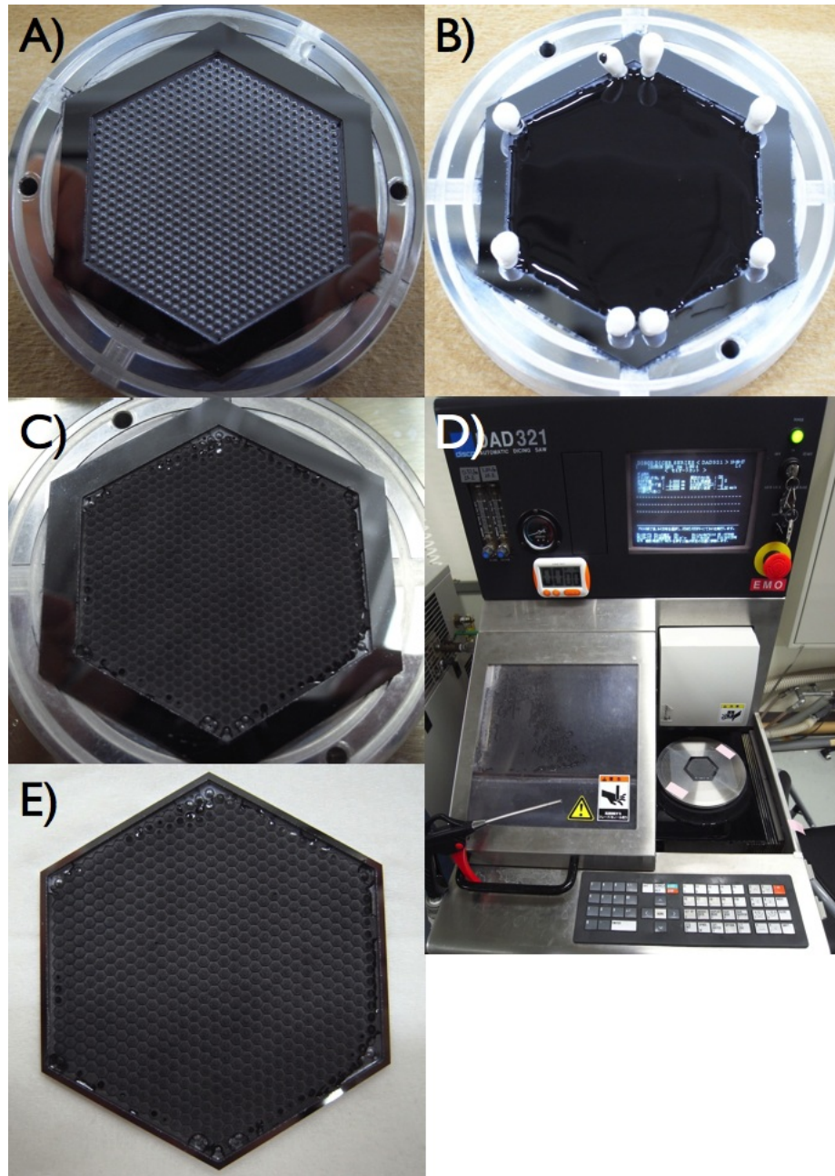
Figure 7.2: (A) Completed 721 pixel silicon lens array in 220-GHz band. (B) The silicon lens array before AR coating fabrication. The lens array was covered with a Stycast epoxy for AR layer. The white pillars protected the alignment holes. (C) The silicon lens array after AR coating fabrication. (D) The photograph of the dicing machine, DAD321, for cutting the edge of the lens array. The lens array was placed on the working table. (E) Completed 721 pixel silicon lens array with single-layer AR coating.
