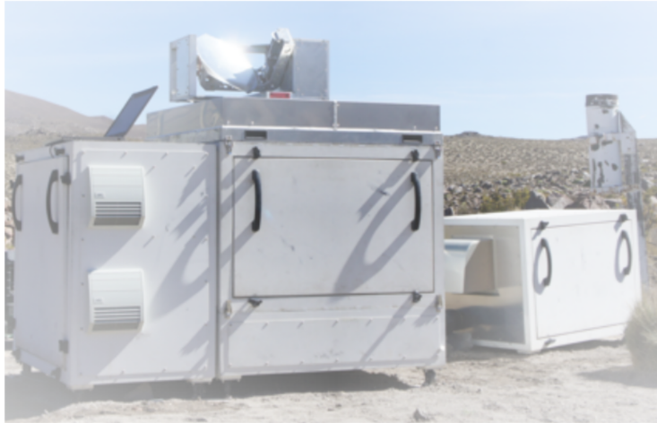
Figure 1.5: Tsukuba 30 cm submillimeter-wave telescope
