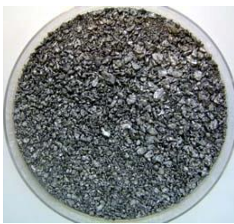
Fig. 3.20 Photographs of solidified fragments and distribution of fragment diameters.
