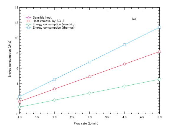
**Fig. 10.** Effect of flow rate on the energy consumption of the cryogenic CO<sub>2</sub> capture system. (a) Pre-chilling stage; (b) CO<sub>2</sub> anti-sublimation stage; (c) storage stage. The temperature of SC-1, 2 and 3 are set at -30°C, -120°C and -120°C, respectively. The COP of SC-1, 2 and 3 are 1.1, 0.7 and 0.7, respectively. The concentration of CO<sub>2</sub> is set at 13%. The conversion efficiency from electric power to thermal energy is defined as 40%.
