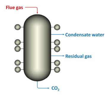
Fig. 14. Conceptual design of the scaled up cryogenic CO<sub>2</sub> capture process based Stirling coolers.
