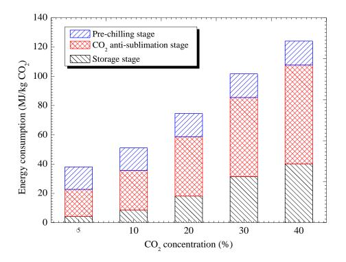
Fig. 11. Influence of  $CO_2$  concentration on the energy consumption of the pre-chilling,  $CO_2$  anti-sublimation and storage stages.
