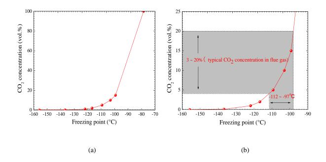
Fig. 2. The relationship between freezing point (°C) and  $CO_2$  concentration (vol.%) (a); in the case of typical flue gas (b).
