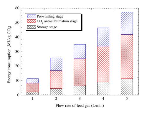
**Fig. 9.** Influence of flow rate on the energy consumption of the pre-chilling, CO<sub>2</sub> anti-sublimation and storage stages.
