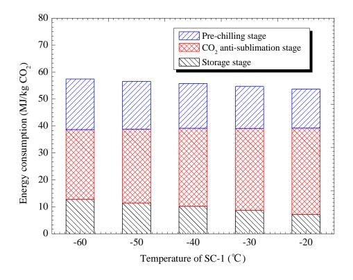
Fig. 7. Influence of temperature of SC-1 on the energy consumption of the pre-chilling,  $CO_2$  anti-sublimation and storage stages.
