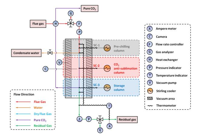
Fig. 1. Schematic of the developed anti-sublimation capture process.
