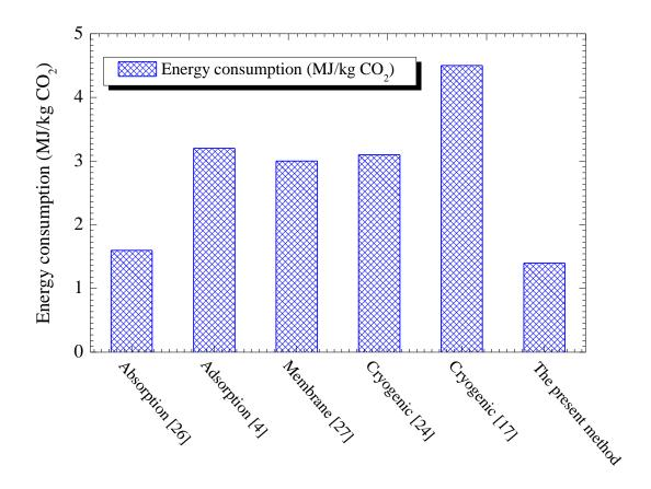
Fig. 13. Comparison of the existing CO<sub>2</sub> capture technologies.
