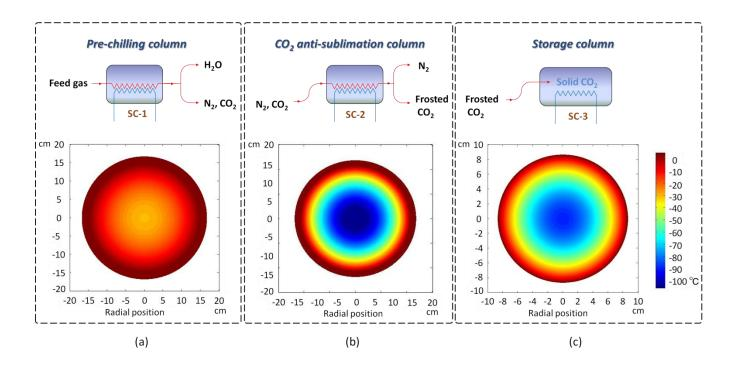
Fig. 5. Temperature distributions in the pre-cooling tower, CO<sub>2</sub> anti-sublimation tower and storage
