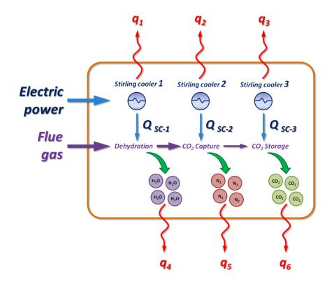
**Fig. 6.** The overall energy flow of the cryogenic  $CO_2$  capture process.
