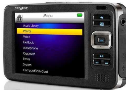
Figure 1.5: Examples of electronics parts utilizing the light-weight of magnesium alloys (9)
