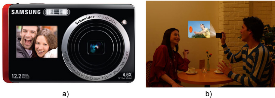
Figure 2.1: Types of cameras. a) Front facing LCD screen camera. b) Projector camera.
