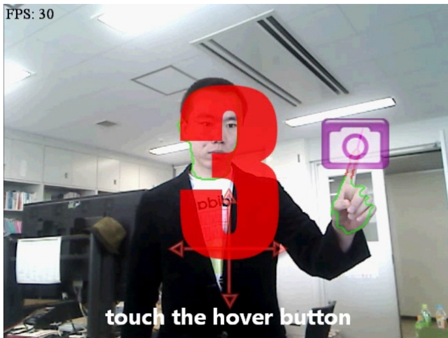
Figure 2.6: The timer will be triggered by the “air touch” of the hover button. After the timer counts down to 1, a picture will be taken.
