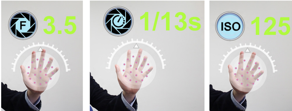
Figure 3.9: Value adjusting interface. Perform circling gesture inside the tracking point circle to adjust the value.
