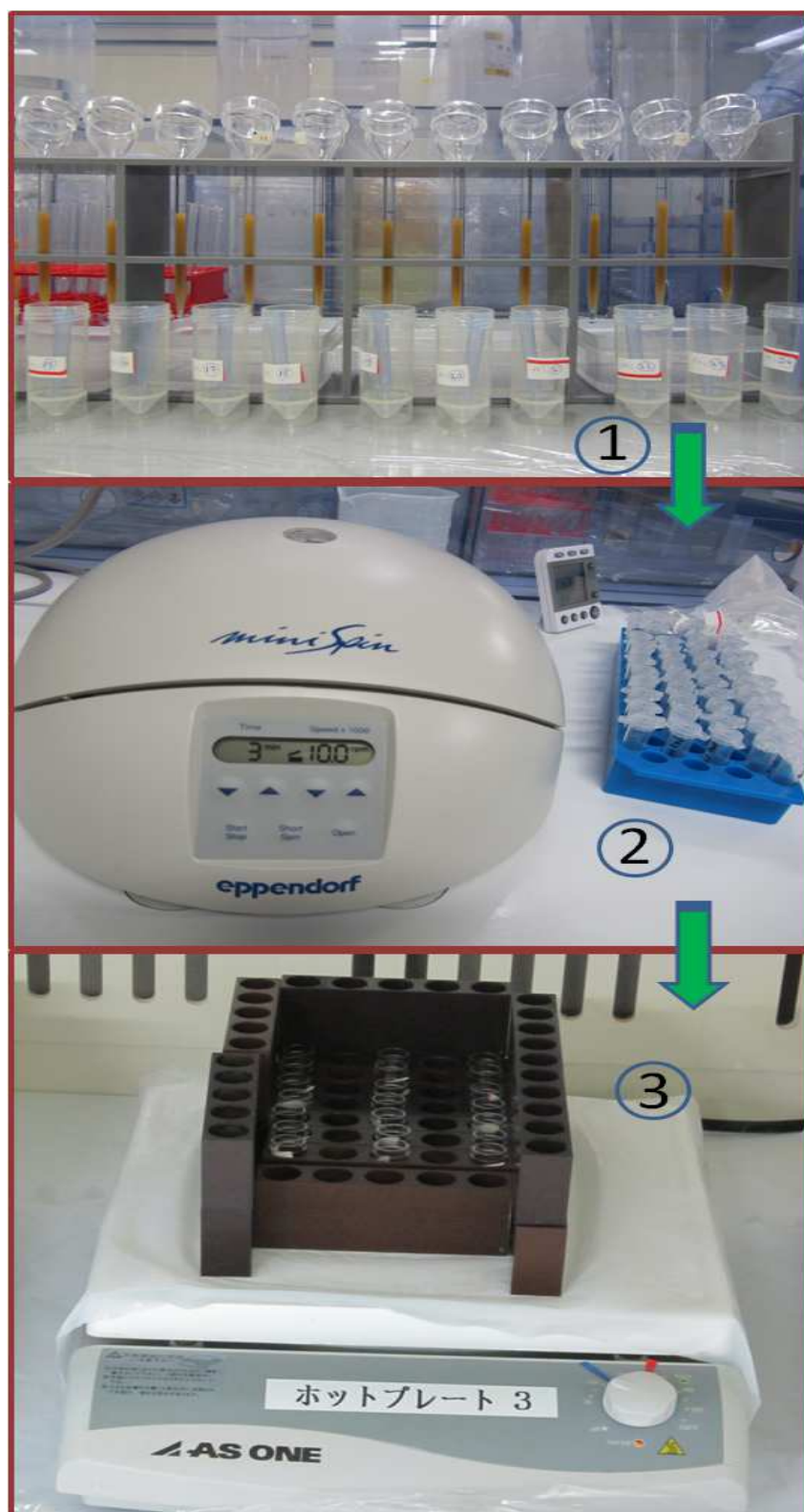
Fig. 3.5 Experiment setup used for strontium isotope analysis (1. Column experiment 2. Centrifugation, 3. Drying at hot plate for overnight)
