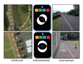
Fig. 8 Field data collection and validation of the results with smart phone
