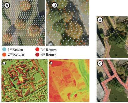
Fig. 4 Manual collection of ground hitting points from DSM to modify original DTM (A & B: 2nd, 3rd and 4th returns are more prominent in edge of the trees whose signals are returning from the ground, C: Shaded DSM, and D: Shaded DTM
