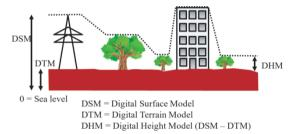
Fig. 1 Illustration of DSM, DTM and DHM in LIDAR data processing
